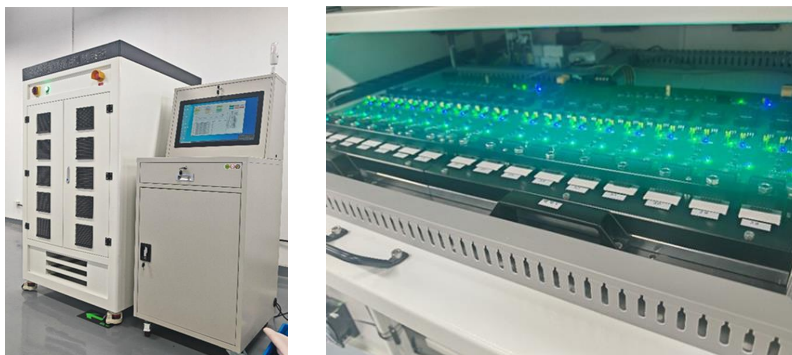
Fig. 2: The DGS Tester (PSL-DHTGB-Pro) and the DUTs mounted inside the DGS tester.
