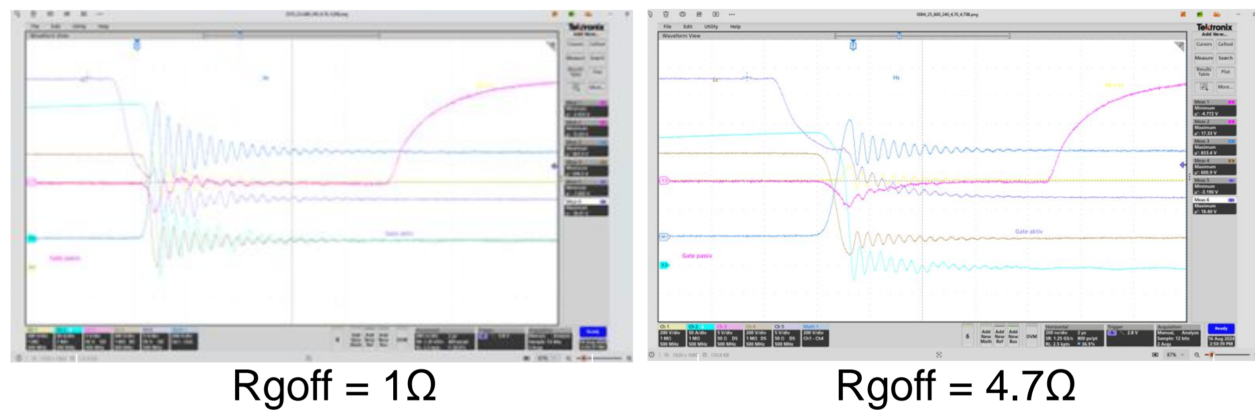
Fig. 3. Relationship between the turn-off resistor parameters and turn-off voltage spikes
