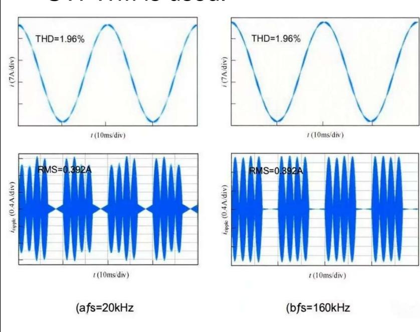
TLI are commonly used in scenarios such as highpower photovoltaic power plants, where the actual power factor is close to the unit power factor, so the maximum frequency can be increased up to 8 times. This constraint specifies the key boundary conditions for high-frequency design.
